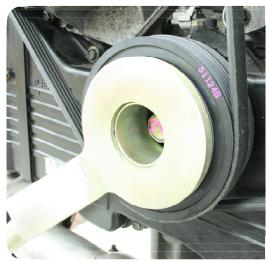
Crankshaft tool fit firmly onto OE damper
